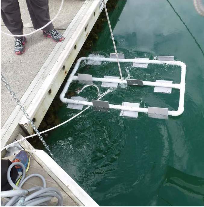
Figure 4 Example of a standard settlement array showing square plates attached to a frame
